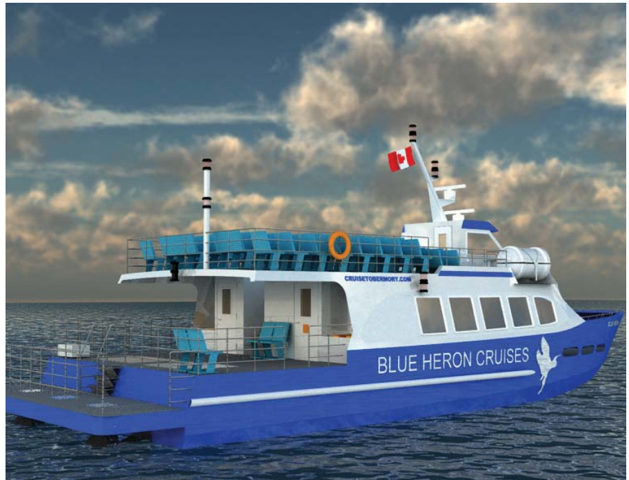
E.Y.E. Marine designed this glass bottom, triple water-jet propelled boat for tours around Georgian Bay’s Flowerpot Islands.
